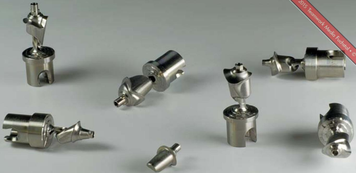
**13** An overview of the customised titanium abutments milled in the Ceramill Motion 2 in the rotational technique. As the blanks are not fixed in position via the precisely prefabricated implant connection geometry there is no impairment of the fit or even damage to be expected in this case
