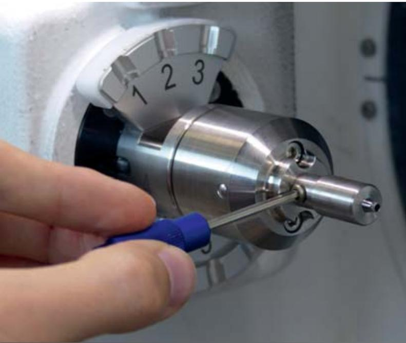
**11** The Preform blank is screwed together with the blank holder of the machine and is thus both concentrically and axially aligned
