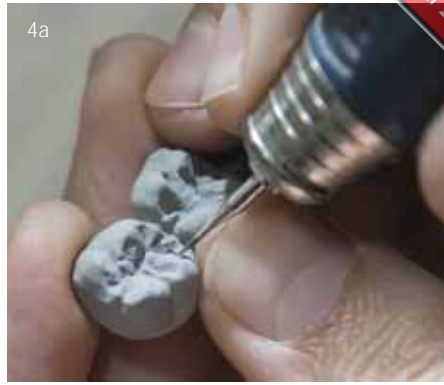
Fig. 3a and 4a First step of customised reworking after dry milling in the Ceramill Motion/Motion2: Fissures and other details can be prepared in the unsintered state using a tungsten carbide cutter (old), which has been tapered using a diamond disc
