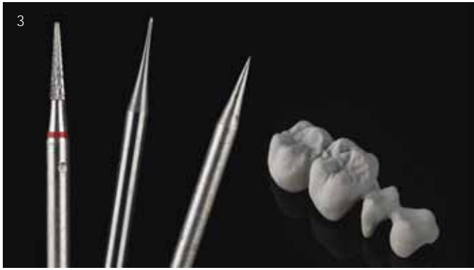
Fig. 3a and 4a First step of customised reworking after dry milling in the Ceramill Motion/Motion2: Fissures and other details can be prepared in the unsintered state using a tungsten carbide cutter (old), which has been tapered using a diamond disc
