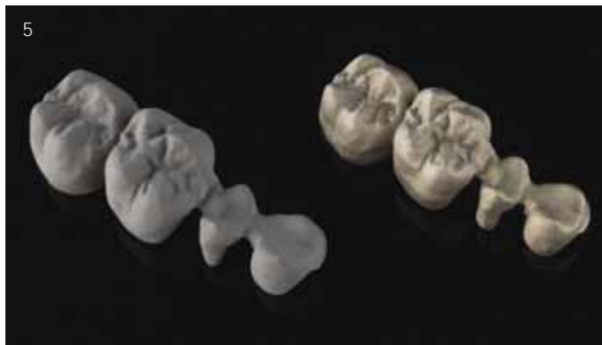
Fig. 5 In the left of the picture the bridge separated from the Ceramill Sintron blank before sintering and after sintering in the right of the picture. The material shrinks by 11 percent during sintering
