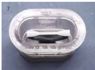
Fig. 7 The milled wax test pieces are sprued and placed in a casting ring for investing
