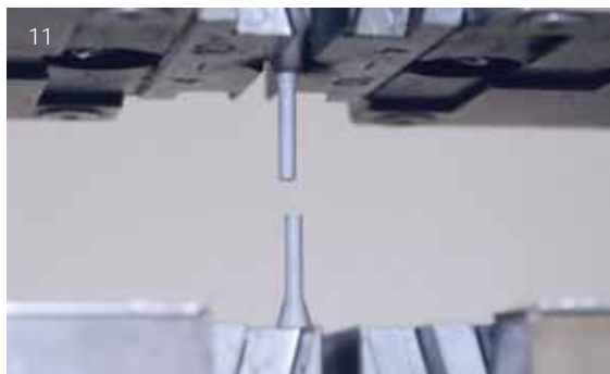
Fig. 11 One of the test pieces after the tensile test. The test piece was pulled apart at a feed rate of 1.5 mm/min. until fracture
