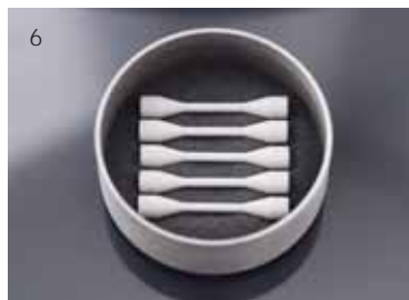
Fig. 6 The Ceramill Sintron tensile test pieces are supported on a layer of sinter beads for sintering
