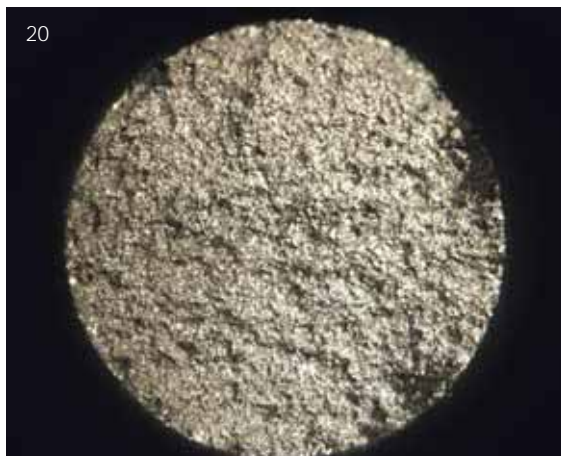
Fig. 20 Light microscopic image of an example of a Ceramill Sintron fracture surface (25x magnification) with homogeneous structure
