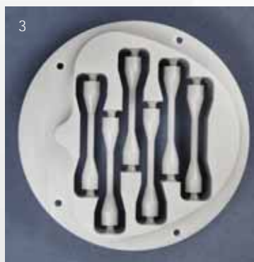
Fig. 3 Tensile test pieces in the wax blank. After separation, the test pieces were sprued, invested and cast using Girobond NB
