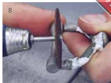
Fig. 8 After cooling, the castings are devested and the sprues are separated from the test pieces
